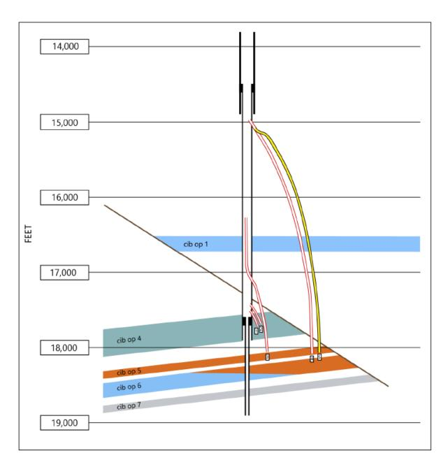
This well was situated in the shallow waters of a bay. Deep beneath that bay at more than three miles below sea level were several natural gas reservoirs, which were known in the region as Cib Op sands.<sup>3</sup> These sands were all separated by layers
